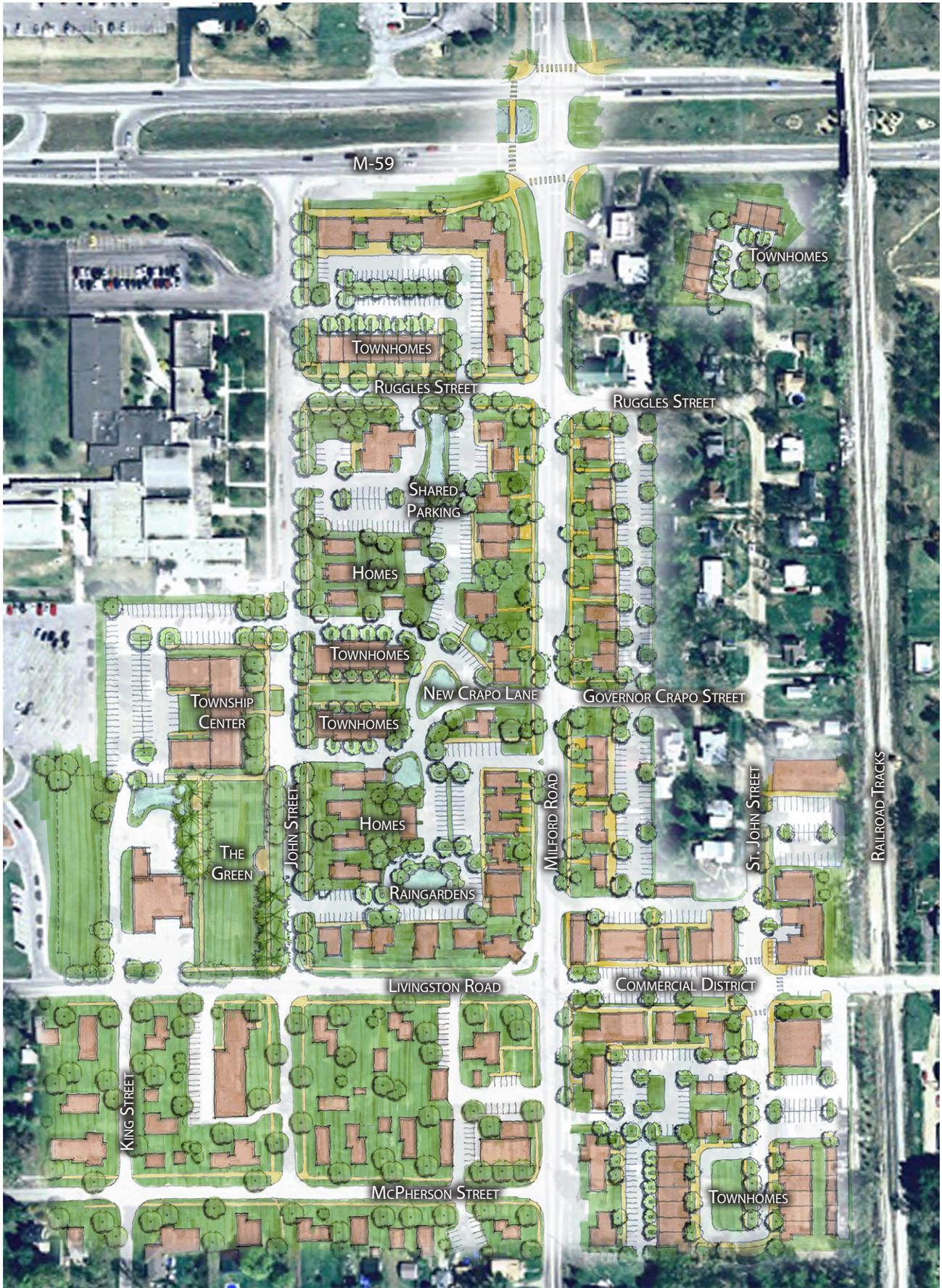
*The Master Plan shows how new roads, buildings, sidewalks, open spaces, and parking lots can be developed to fulfill the goals of the Highland Station Vision and Framework Plans.*
