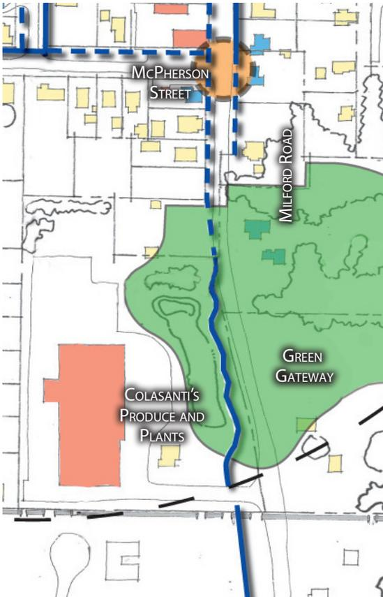
*A plan for pedestrian connections to the Green Gateway shows sidewalks in blue. Solid lines represent existing sidewalks and dashed lines represent potential connections.*
