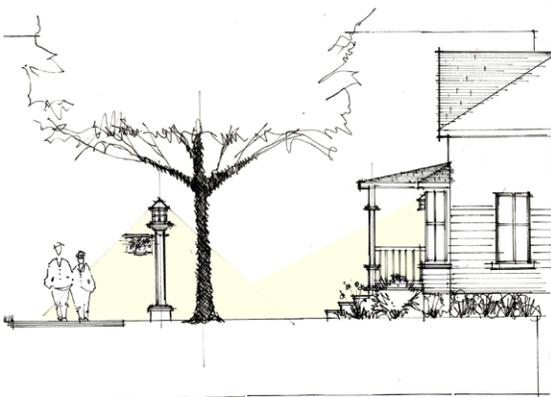
*A section through the front yard of a commercial building shows how porch lights and poles can light sidewalks.*
